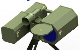
Laser Kill Eyesafe Laser Interceptor is a compact 1kW single mode LWIR laser designed for defense applications. The laser includes up to 500 mm diameter reflective telescope, focusing, tracking and steering optics. The laser is accomplished with a compact laser driver and a chiller. The interceptor is mounted on a precise fast 2 axis tracking stage for rotation of the laser towards targets.
