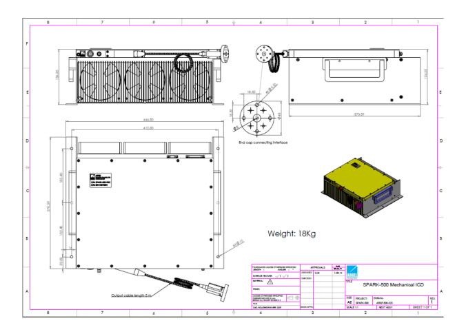
Figure 2: Mechanical drawing of the laser module.
