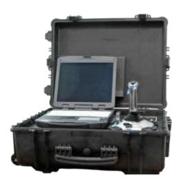
The CITRON is a short to long range electro-optical missile threat simulator for testing missile approach warning systems (MAWS) and for training crew in the operation of these systems.
